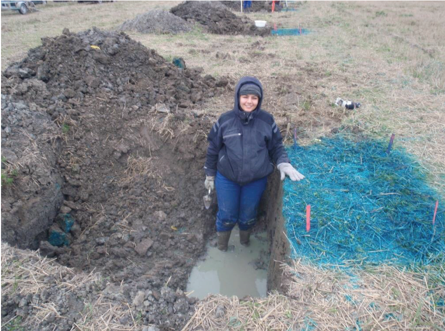
Figure 9. Preparing profile walls for photographing dye pathways during the dye tracing test.
