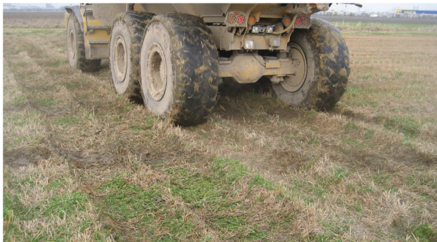
Figure 2. Experimental compaction treatment involving four passes with a 5-ton wheel load dumper truck.
