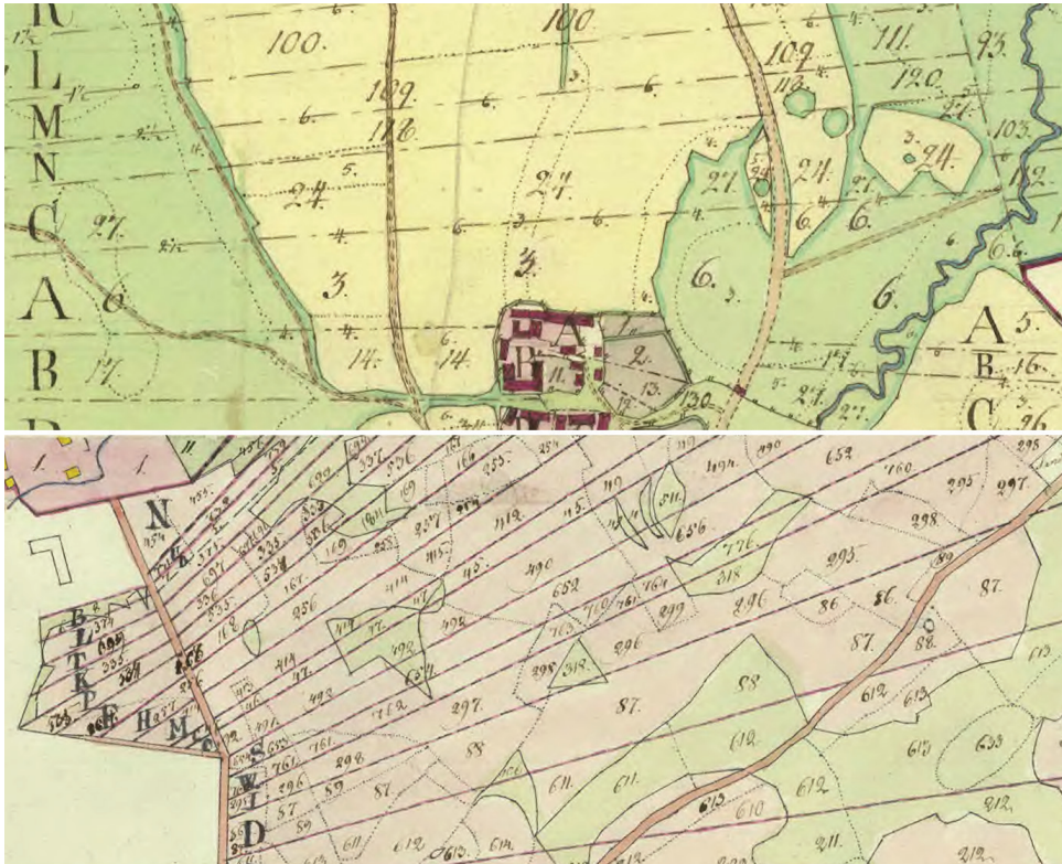
Figure 10 & 11. Above: Detail of the storskifte map of Friggeråker (1800). Below: Segerstad storskifte (1822). In the two surveys the new division and borders between holdings are marked with straight lines with letters referring to which farm it belongs (A, B, C and so on). In Segerstad (below) the number within each new parcel refers to the text section where the soil quality is specified for each number. 'Underneath' the new division, the dotted lines delimit differences in quality. In Friggeråker (above) the procedure is the same, in addition, the surveyor has written the korntal (crop yields) on the map as well. (Source: Friggeråker LSA P54-5:4; Segerstad LSA P175-9:6)
