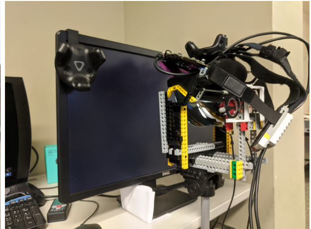
Figure 3.2. Apparatus used to calibrate the AR HMD
