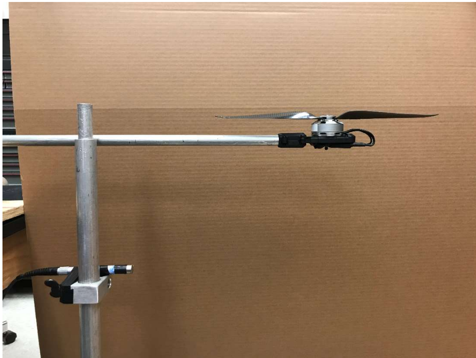
Figure 3.6. Microphone placed 30cm from the far end of the housing and 18cm below the arm.
