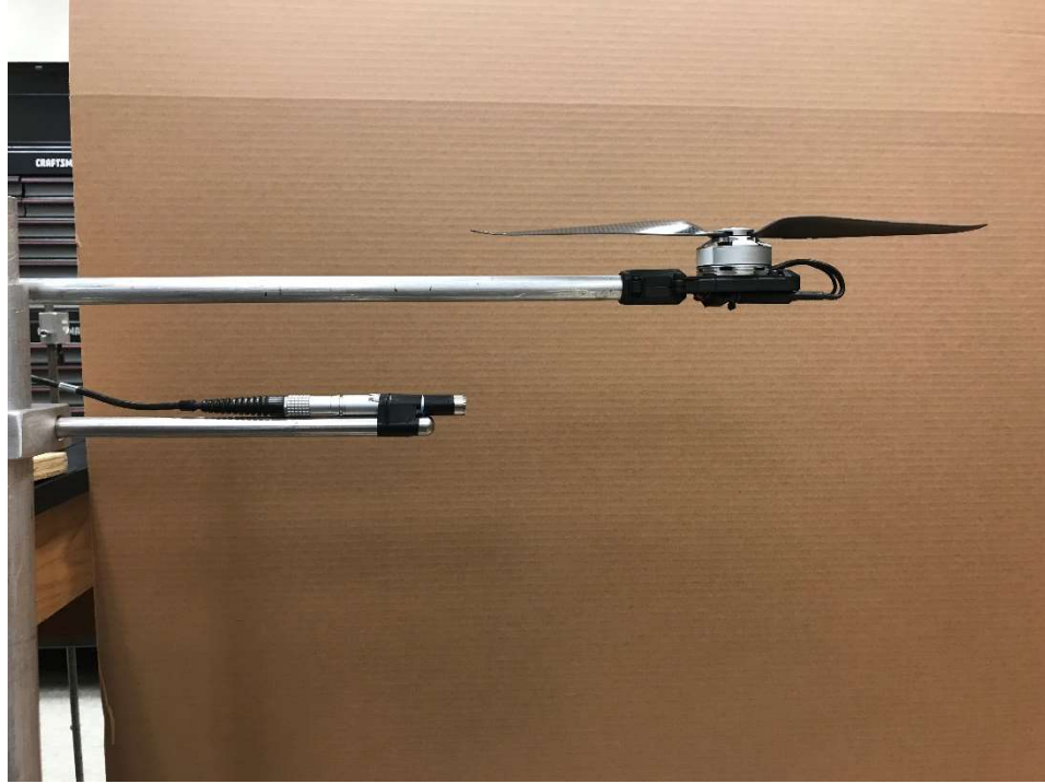
Figure 3.5. Microphone placed 11cm from the far end of the housing and 6cm below the arm.
