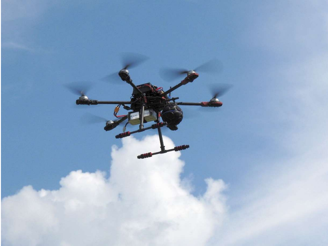
Figure 4.1. Tarot 680 Pro with Zylia ZM – 1 spherical array
