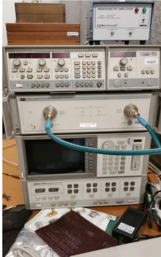
Figure 8: HP 8530A Network Analyzer
