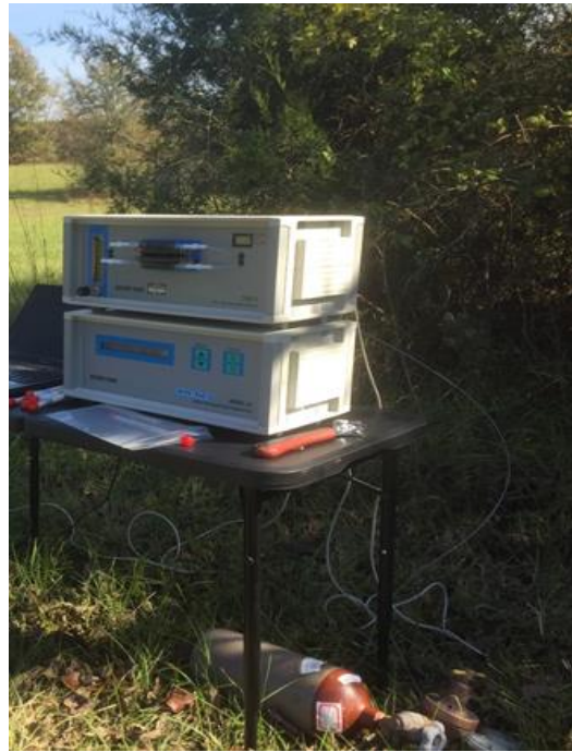
Figure 6. Brooks-Rand TDM-II CVAFS field setup
