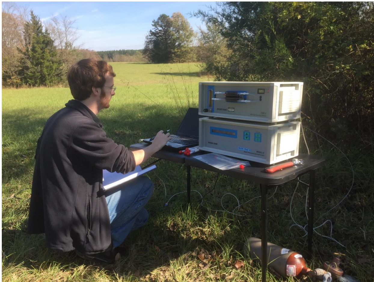
Figure 14. Field analysis of quadcopter-deployed gold-coated Hg traps by CVAFS
