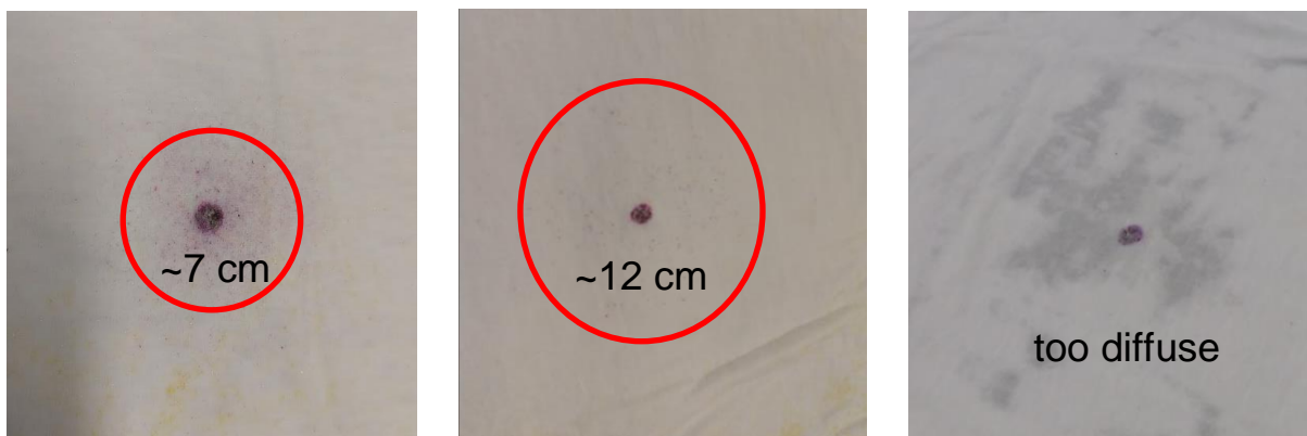
Figure 49. Lead and Nitrite GSR deposition from a .22 caliber Songbird (increasing distance left to right: 0.46m, 0.91m, 1.37m)
