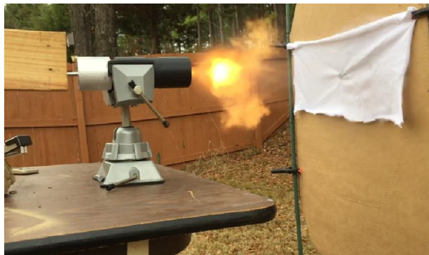
Figure 30. .38 caliber ABS polymer firearm
