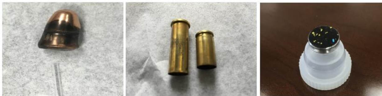
Figure 16. Categories of trace evidence analyzed in this study. Bullet fired from a gun with a black ABS barrel showing a polymer smear mark and scrape marks from the melting point tube used for DART-MS analysis (left). Cartridge case from the same gun (middle, left shell) showing external black polymer residue, unlike a cartridge case from a traditional gun (middle, right shell). Adhesive stub used to collect GSR and occasionally polymer (colored) fragments from a cotton t-shirt (right)
