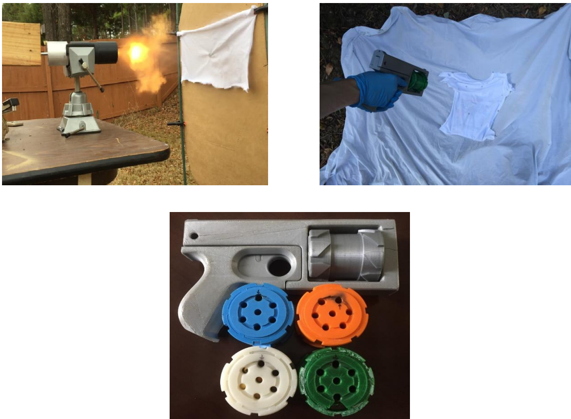
Figure 15. Phase I test-fire of ABS polymer barrel (top left). Fully 3D-printed gun and interchangeable cylinders composed of blue CPE, white ABS, orange PLA, and green PETG (bottom center). Phase II test-fire of 3D-printed gun (top right)
