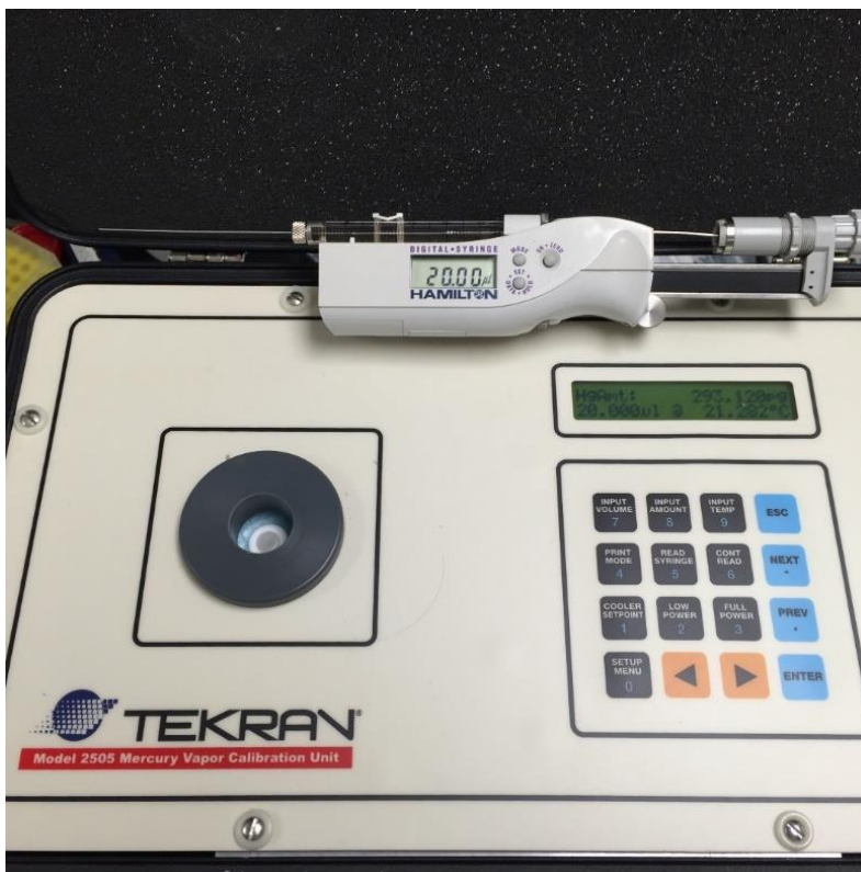
Figure 8. Gaseous Hg calibration unit (Tekran 2505) with digital syringe
