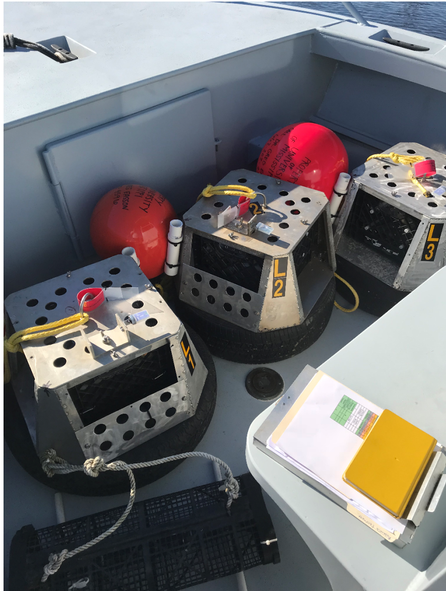
Figure 5: OOS with biosensor rack and abiotic sensors
