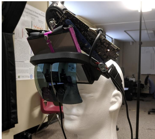
Figure 4: Custom-built optical see-through AR HMD
