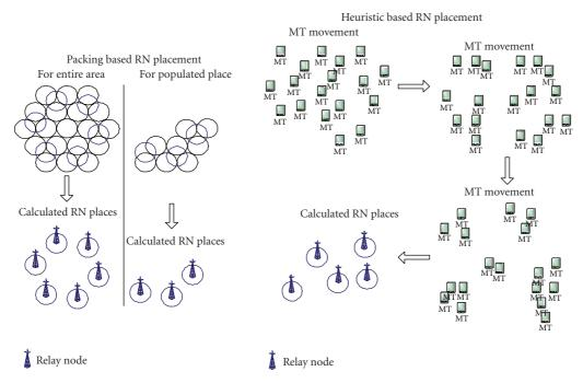
FIGURE 3: Packing-based RN placement and heuristic RN placement.
