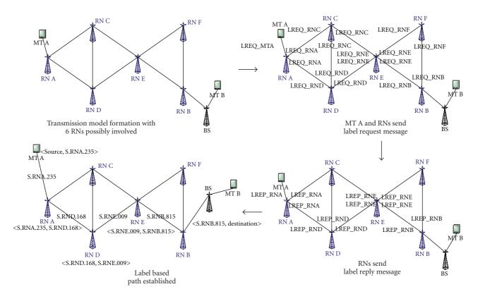
FIGURE 6: Label routing illustration.
