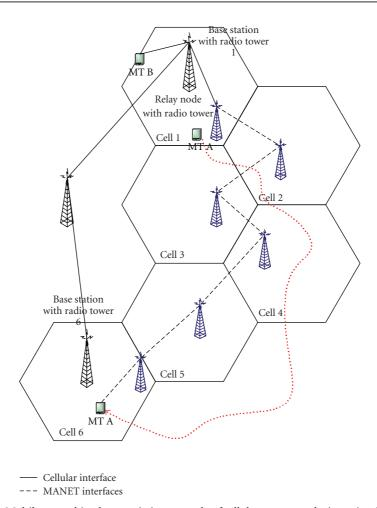
FIGURE 2: Multihop combined transmission example of cellular resource relaying using fixed RNs.
