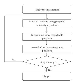
FIGURE 4: Flowchart of heuristic RN placement.
