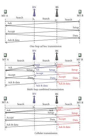
FIGURE 5: Computerised ADCR algorithm and simplified transmission modes illustration.
