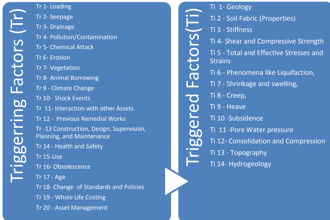
Figure 4.4: List of Triggering and Triggered factors affecting the performance of geotechnical assets
