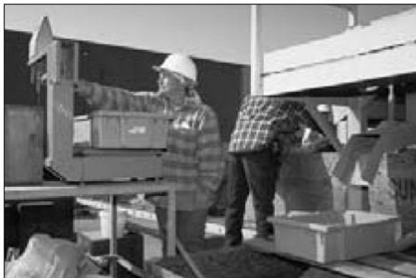
Figure 14. The sand that falls through the agitator is collected when the containers are unloaded. The sand is weighed and the average per container is deducted from the gross weight delivered. Photo: Jack Kelly Clark. Source: Raisin Production Manual. Christensen, 2000.
