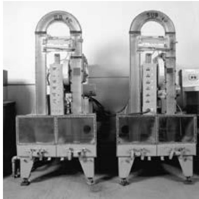
Figure 18. Air current sorting machines are used to determine ripeness and raisin grades: "Substandard" or "B or better". They are put in order using a continuous air flow at a constant temperature and pressure. Photo: Jack Kelly Clark. Source: Raisin Production Manual. Christensen, 2000.
