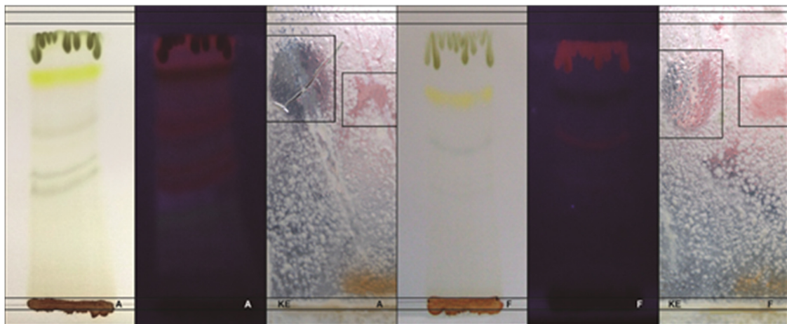
Figure 1. Contact bioautography: Extracts A and F of P. dubium against A. flavus . From left to right: (A), thin layer chromatography (TLC) of P. dubium leaf extract (visible light); UV at 366 nm and contact bioautography. (F) TLC of P. dubium leaf extract (visible light); UV at 366 nm and contact bioautography.
