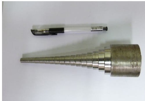
Figure 5.8 The machined aluminium rod with various diameters that was used in the bending test
