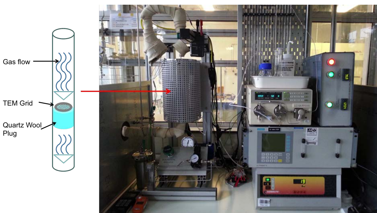
Figure 2.21: Vapour-phase chemical reaction facility. Photo credit to Christopher M. Brown, Johnson Matthey Technology Centre.
