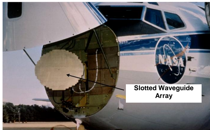
Figure 2.6: A planar array slotted waveguide antenna is used in the radar system in the NASA Boeing plane 737 [8].
