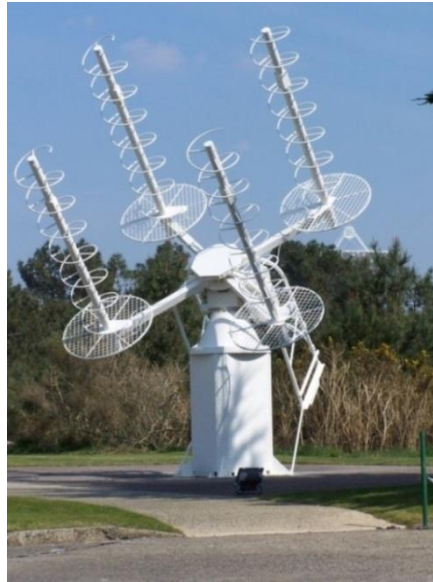
Figure 2.5: An array of four axial-mode helical antennas, France [7].
