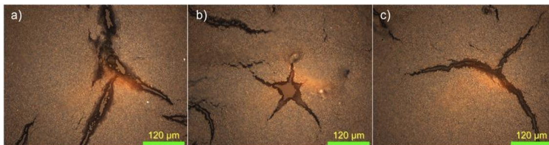
Fig. 6.18 Surface images of the commercial (a) 35BC, (b) 35CC and (c) 35DC GDLs.
