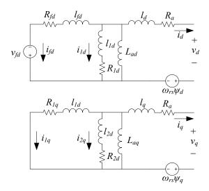
Fig. 3.5 Equivalent circuits of the synchronous machine (above: *d*-axis circuit; below: *q*-axis circuit)
