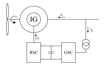
Fig. 3.1 Configuration of DFIG-based wind turbine
