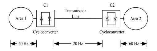
Fig. 6.1 Structure of the FFTS in system interconnections
