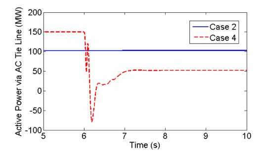
Fig. 6.10 Active power via conventional AC tie line in Case 2 and Case 4
