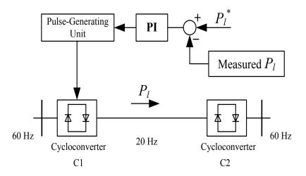
Fig. 6.8 Power flow controller for FFTS
