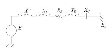
Fig. 2.1. A simple radial series compensated system
