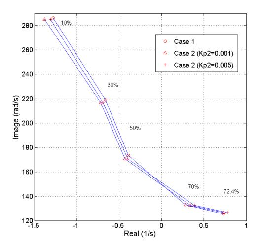
Fig. 4.8 Eigenvalue of network mode under different compensation level for Case 1 and Case 2 with various control parameters
