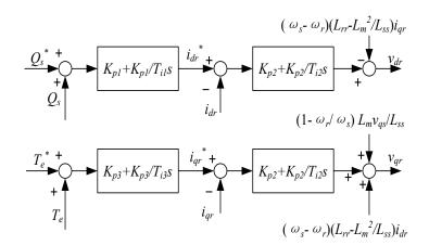
Fig. 3.3 Control block diagram of rotor-side converter
