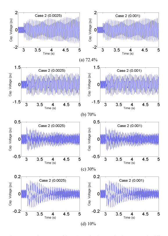
Fig. 4.7 Dynamic response of the voltage of series capacitor in Case 2 under different control parameters
