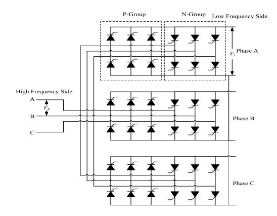
Fig. 5.3 Structure of a three phase cycloconverter
