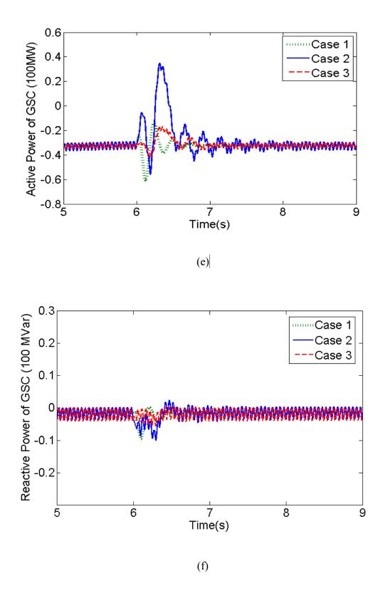
Fig. 5.5 Dynamic responses for Case 1, 2 and 3 in SMIB under fault
