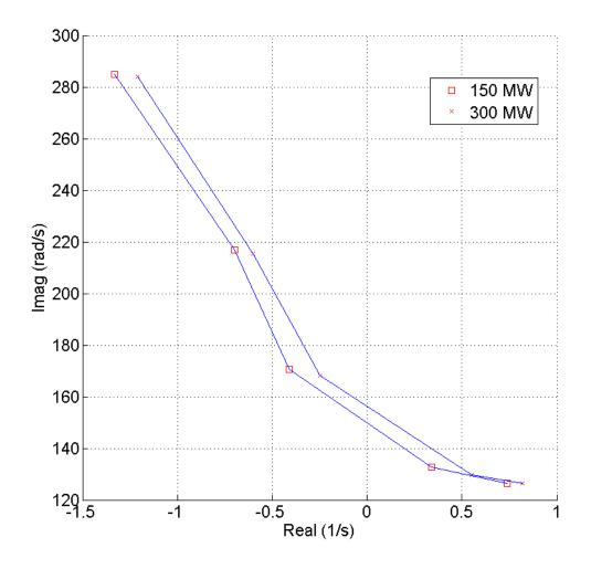
Fig. 4.10 Network resonance mode under different compensation level for Case 2 with increased wind farm scale
