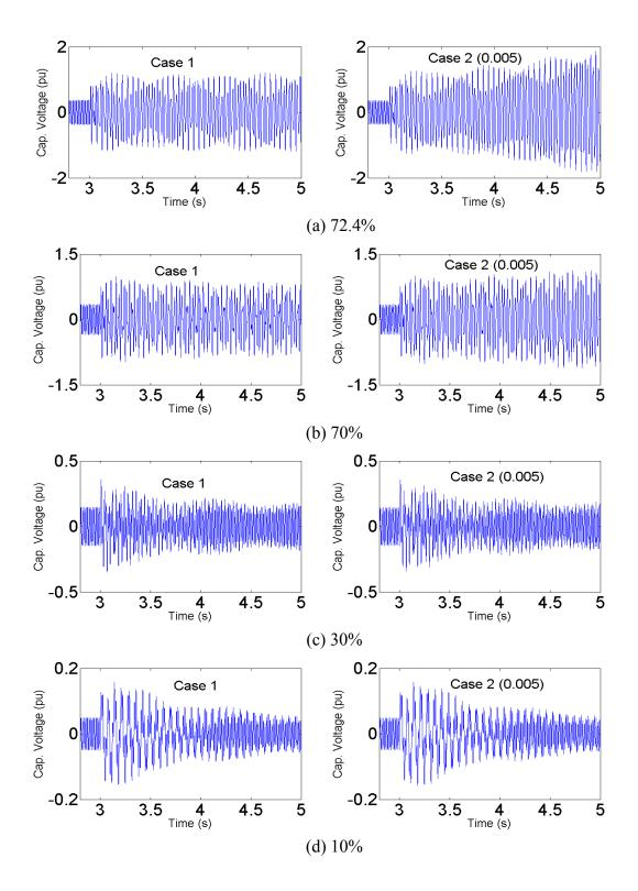
Fig. 4.6 Dynamic response of the voltage of series capacitor in Case 1 and Case 2 ( $K_{p2}$ = 0.005)
