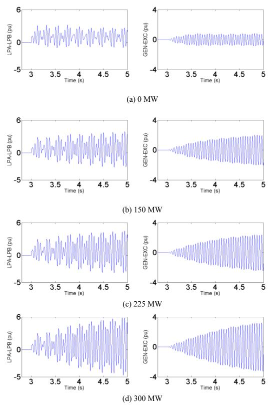
Fig. 4.3 Torsional response of Mode 2 with (a) 0 MW, (b) 150 MW, (c) 225 MW and (d) 300 MW wind farm
