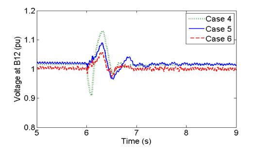
Fig. 5.9 Voltage responses at Bus B12 for Case 4, 5 and 6 under fault
