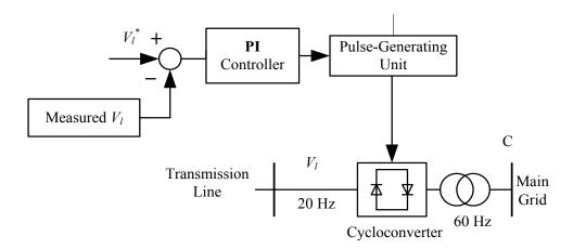
Fig. 5.4 Feedback control loop for cycloconverter
