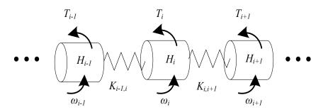
Fig. 3.6 Shaft system of the T-G unit
