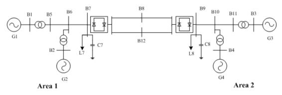
Fig. 6.4 Configuration of Case 3
