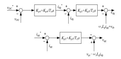
Fig. 3.4 Control block diagram of grid-side converter
