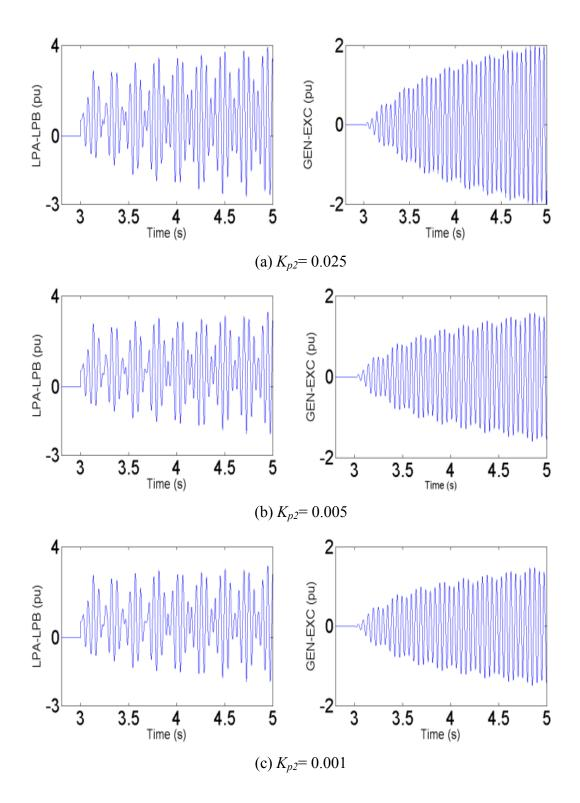
Fig. 4.4 Torsional response of Mode 2 under different  $K_{p2}$
