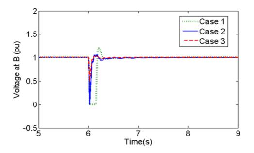
Fig. 5.6 Voltage dynamics at Bus B for Case 1, 2 and 3 under fault
