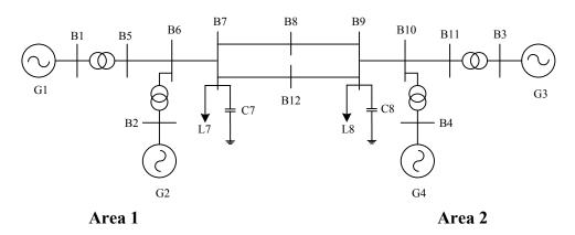
Fig. 6.2 Two-area system (Case 1)
