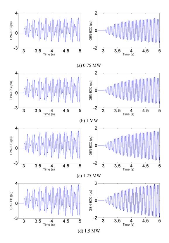
Fig. 4.5 Torsional response of Mode 2 under different operating point
