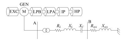
Fig. 4.1 IEEE first benchmark model for SSR analysis
