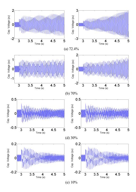
Fig. 4.9 Dynamic response of series capacitor voltage in Case 2 (225 MW) and Case 2 (300 MW)
