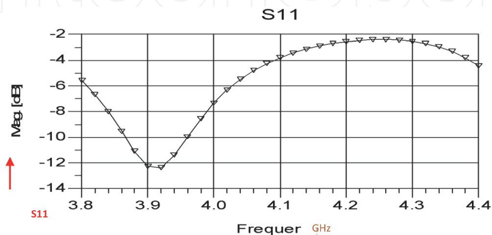
Figure 26. Computed S11 of the microstrip stacked patch.
