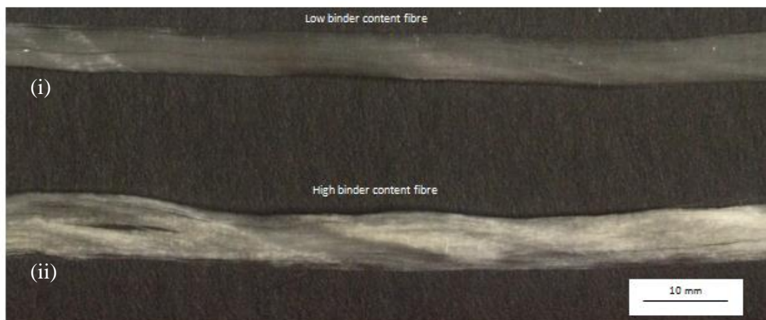
Figure 4.71 A photograph showing (i) low; and (ii) high binder content in Type-I fibres.
