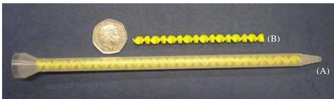
Figure 2.12 A photograph showing (A) a static mixer and (B) the helical inner element (Shotton-Gale, 2013)
