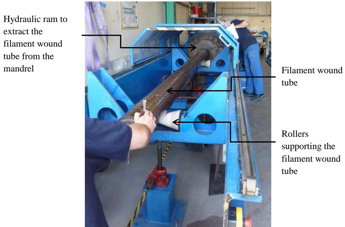
Figure 3.9 A photograph showing the hydraulic ram used for mandrel extraction.
