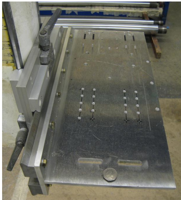
Figure 4.32 The interface platform that was used to mount Prototype-1 and Prototype-2 to the industrial filament winding machine (A) A detailed schematic of the interface platform. (B) A photograph showing the interface platform mounted on the filament winding machine.
