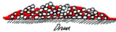
Figure 4.3 A schematic illustration of the observed impregnation at contact point-(ii) in Figure 4.1.
