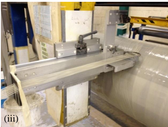
Figure 3.2 Photographs showing: (i) Pre-tension device; (ii) Resin bath; (iii) Traversing platform; and (iv) D-eye.
