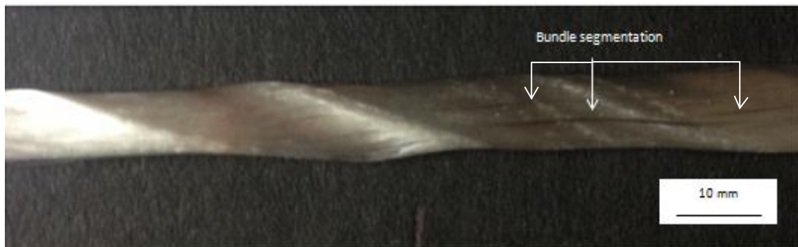
Figure 4.70 A photograph of Type-II fibres showing typical splitting/segmentation of the fibre bundle.
