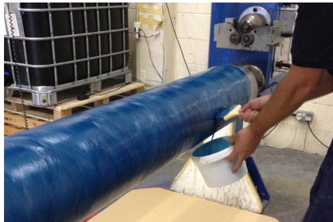
Figure 4.13 A photograph showing the manual intervention carried out on a 10 inch diameter mandrel during conventional filament winding to remove the excess resin and/or to impregnate the under-impregnated areas.
