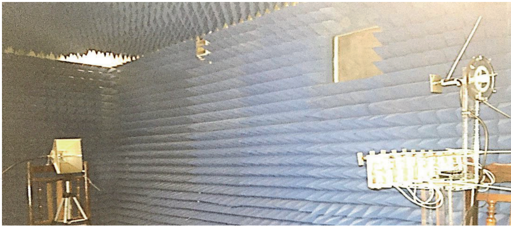
Figure 31. Array antenna measurement in anechoic chamber.
