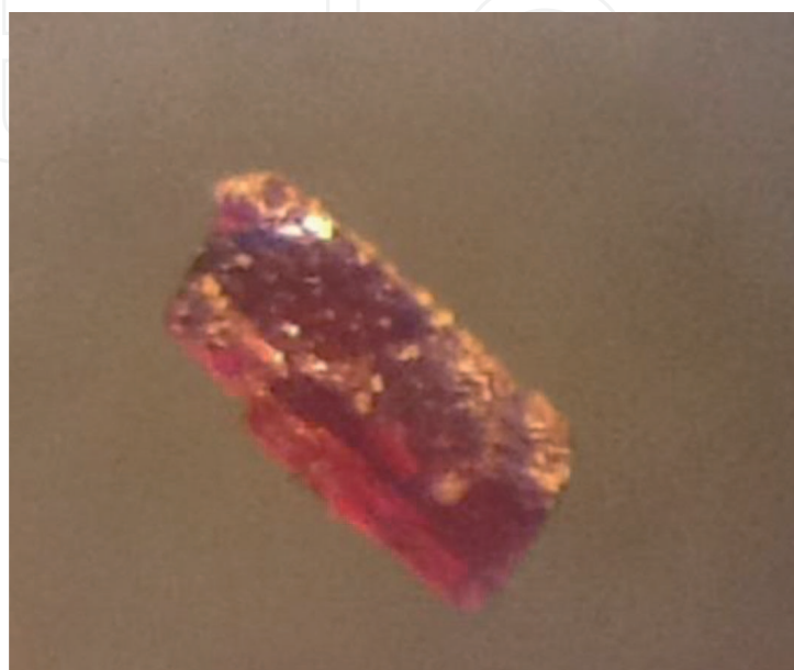
Figure 2. Image of a single crystal of the phase \text{Na}_{1.25}\text{Co}_{2.187}\text{Al}_{1.125}(\text{AsO}_4)_3 [9] seen under the binocular magnifying glass.
