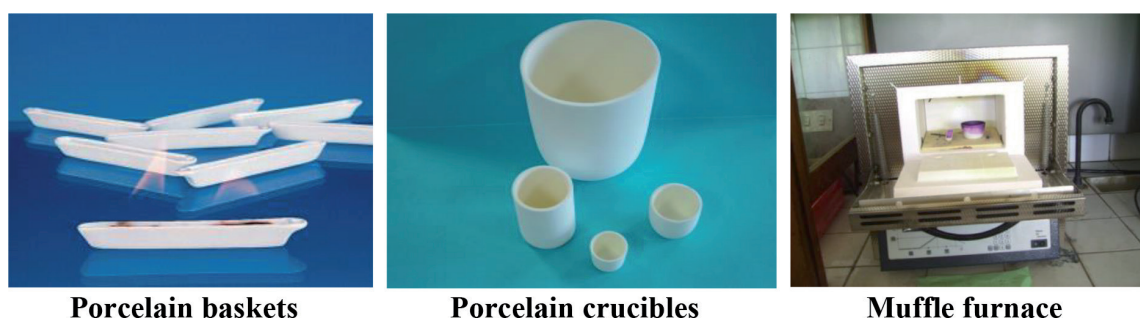
Figure 1. Equipment used in solid-state synthesis.
