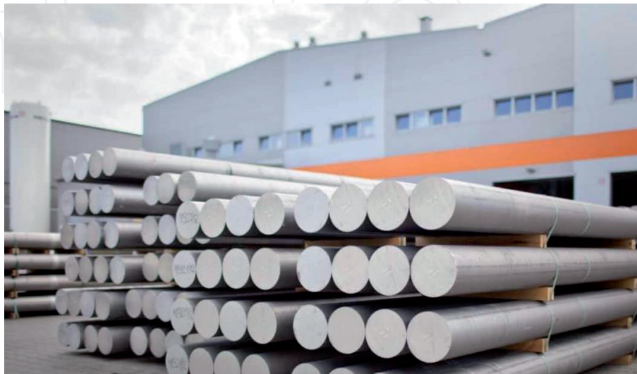
Figure 8. Aluminum alloy billets before loading onto the loading ramp of the press [26].
