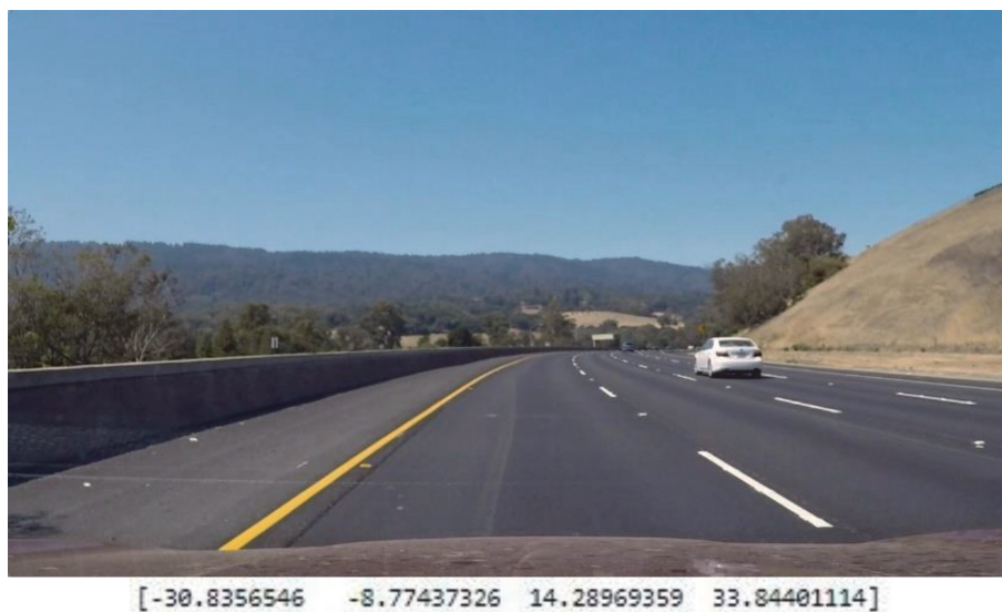
Figure 3. The image that edge distribution function generated from and local maxima points. Local maxima points on edge distribution function are detected and within these points, the possibility of being lane boundaries of the center lane is found as a result of thresholding.
