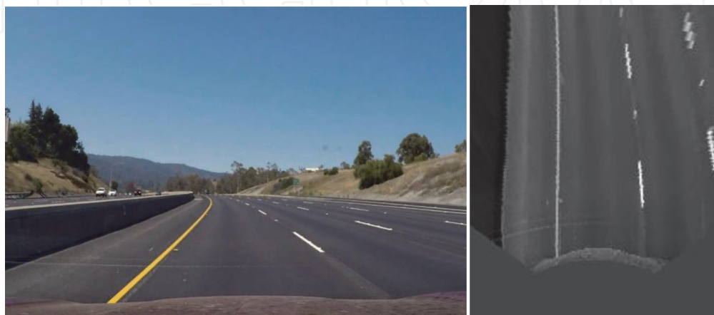
Figure 8. Inverse perspective mapping example. Average camera parameters for bird view image of the original image (left) manually selected and bird view image (right) is found. The original image size is (720, 1280) and the bird view size is (200, 200).
