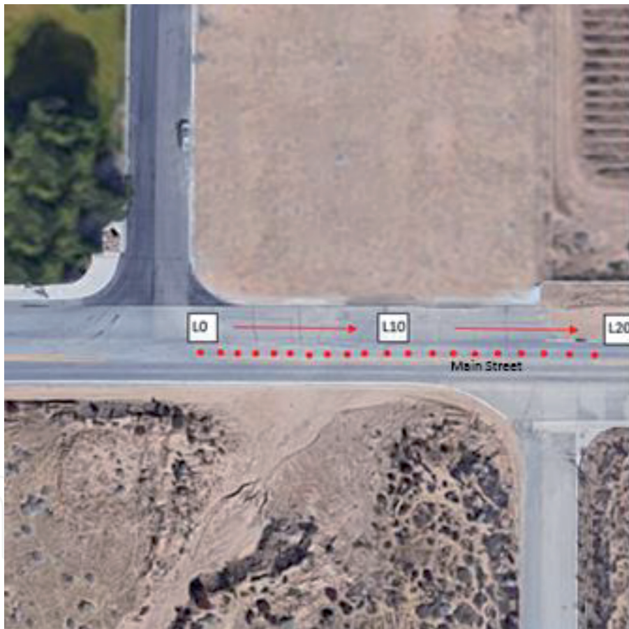
Figure 5. Location of the probes along the center of the main street. The flow depth results were compared at probe locations 9 and 13.
