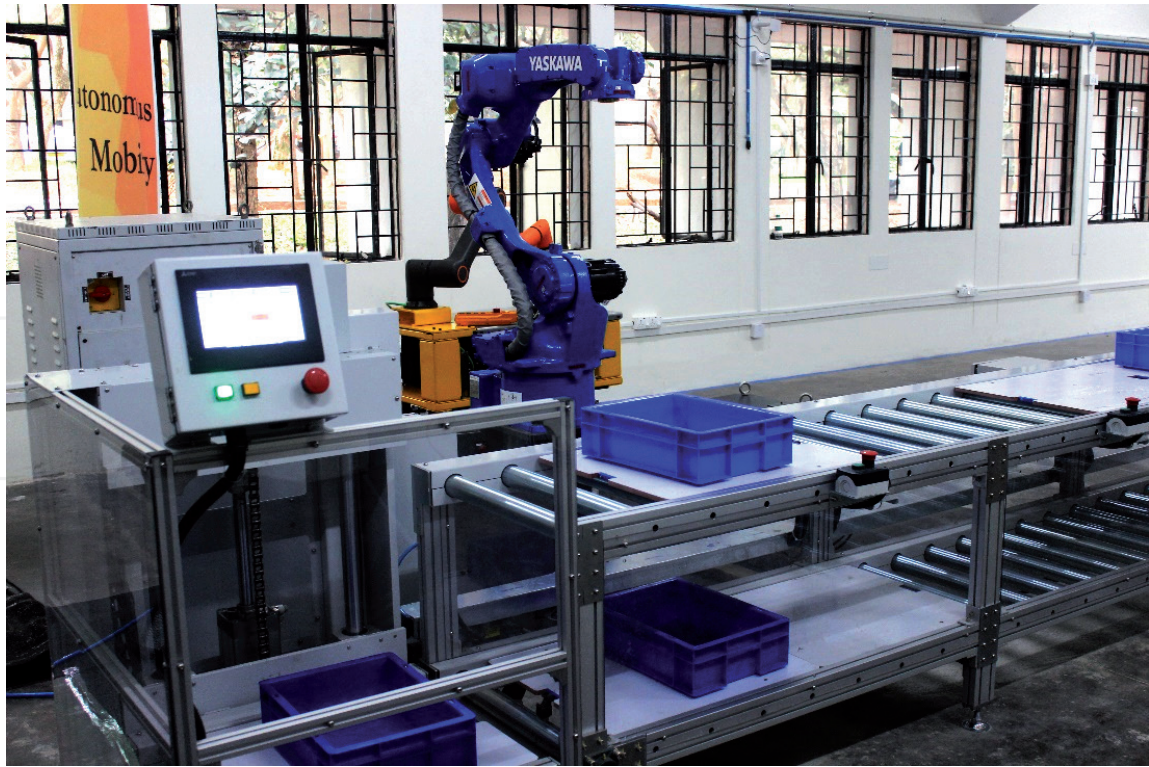
Figure 3. Yasakawa Robotic arm used for to pick and sort different items from a conveyor.
