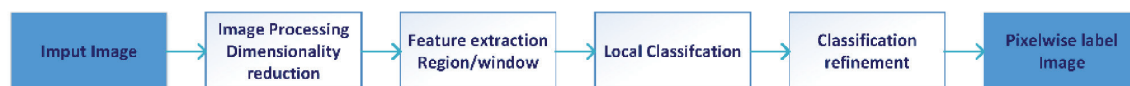
Figure 3. Block diagram of a classical architecture approach for semantic segmentation using computer vision.
