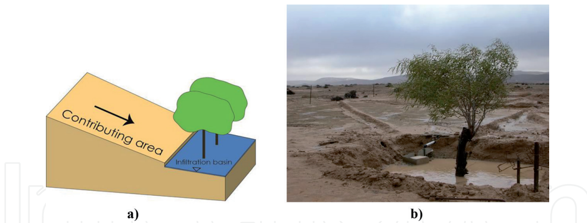
Figure 6. Traditionally designed micro-catchment system: (a) schematic of the system and (b) flooded micro-catchment.
