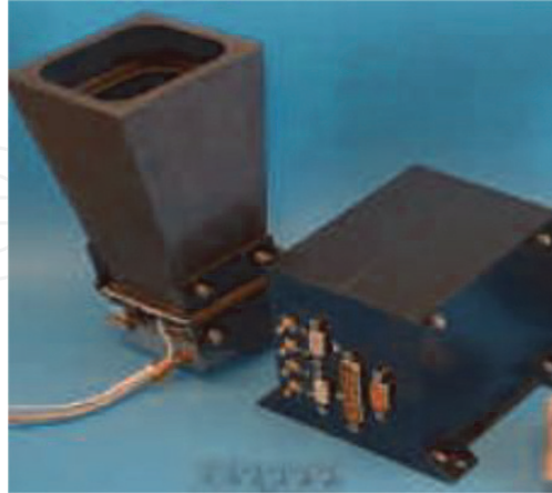
Figure 13. Star direction R -vector measured sensor (optic and computer units). Advanced stellar compass, accuracy, 2'' - 16'' ( 2\sigma ).
