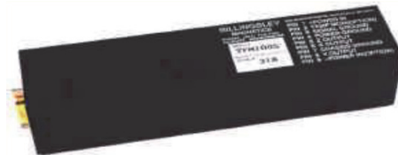
Figure 12. B-vector sensor MAG TFM100-S, accuracy, 10mG ( 2\sigma ).
