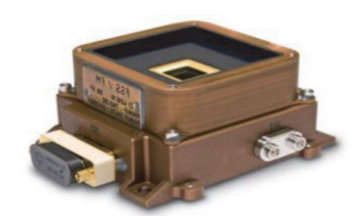
Figure 10. S-vector sensor Bradford fine sun sensor, accuracy, 0.2 deg. ( 2\sigma ).
