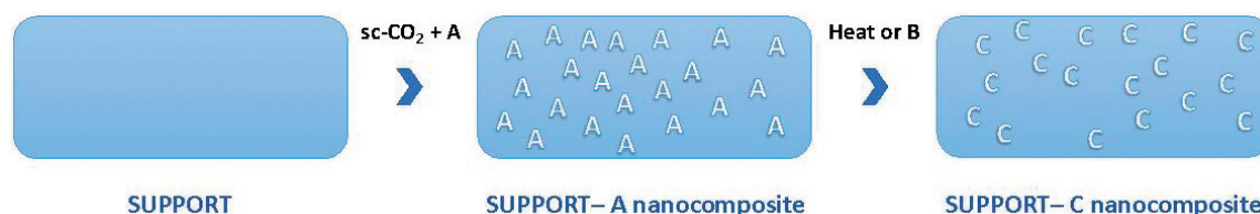
Figure 4. Schematic diagram for supercritical fluid deposition method. (a) Organometallic precursor, (b) reducing agent, and (c) metal nanoparticles.
