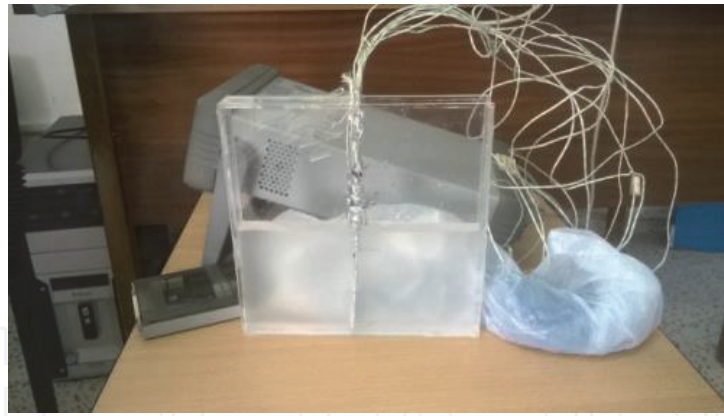
Figure 2. PCM wall filled with Paraffin-27.
