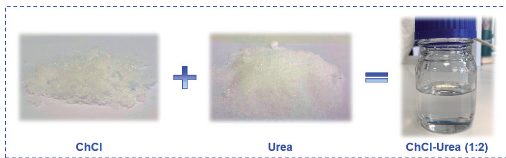
Figure 4. Choline chloride, urea, and clear liquid DES of ChCl-urea (1:2).
