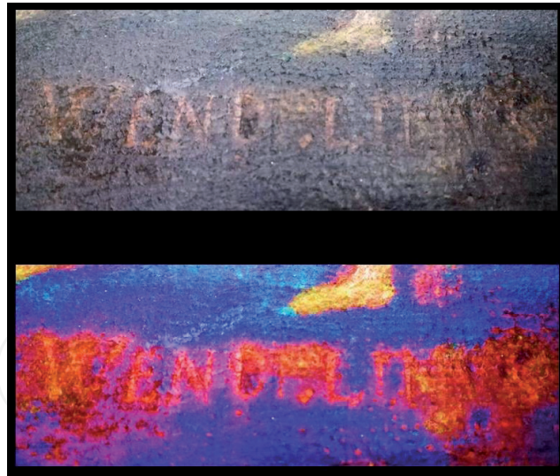
Figure 10. The ultraviolet light analysis for the signature WENDELINUS.
