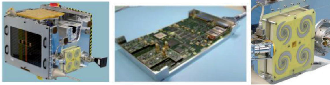
Figure 10. (Left) TechDemoSat-1 (TDS-1) prior to launch (Centre) SGR-ReSI SGR-ReSI, part of sea-state payload on TDS-1 (Right) TDS-1 nadir GNSS antenna [14].
