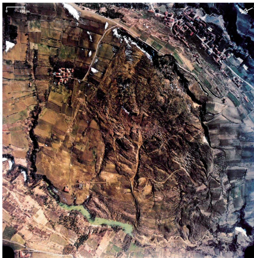
Figure 5. Aerial photograph of the huge translational rock-block slide at Somano (February 1974). The movement stopped at the opposite slope causing a dam and consequent small lake of the Gamba stream.
