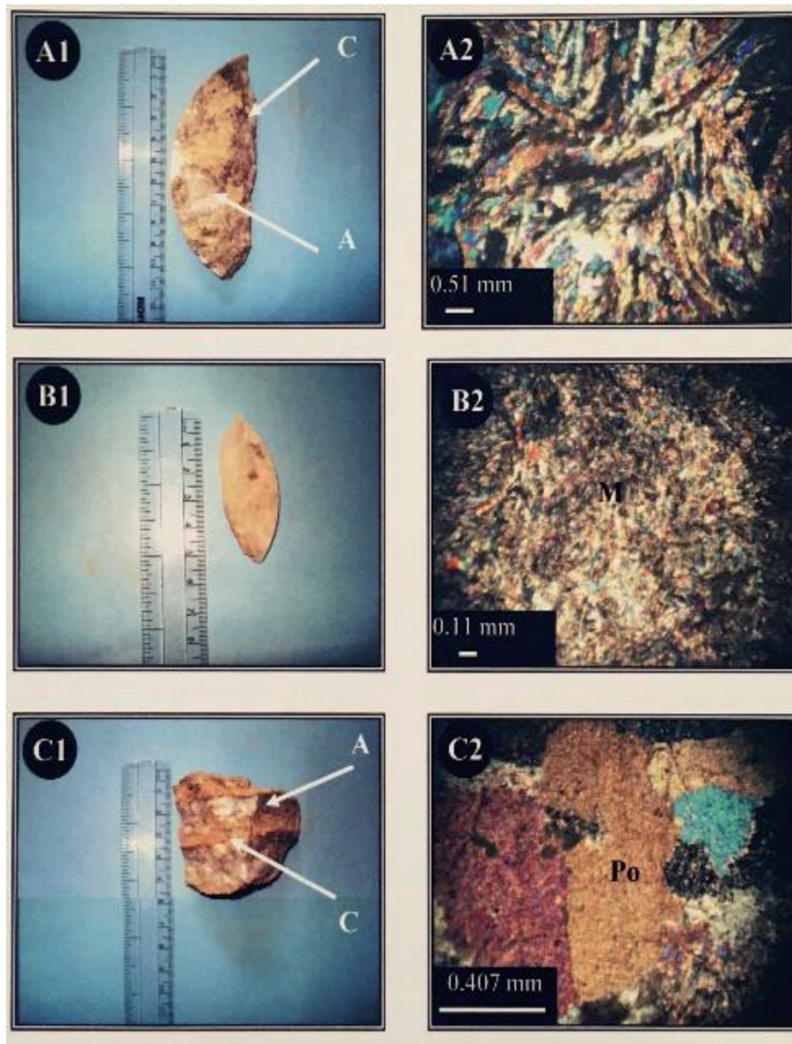
Figure 10. (A1) Fine anhydrite nodule (A) in carbonate specimen (C), Kirkuk well; (A2) thin section of the same sample in A1, showing flow structures in anhydrite; (B1) finely crystalline anhydrite nodule, Kirkuk well; (B2) thin section for the same sample in B1 showing microcrystalline texture; (C1) finely intercalations of anhydrite nodules (A) and carbonates (C), Kirkuk well; (C2) thin section of the same sample C1 showing porphyroblastic texture (Po).
