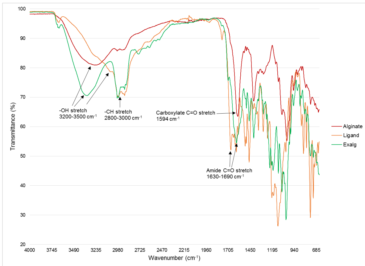
Figure 26 IR spectra of alginate, ligand 33 and Exalg .
