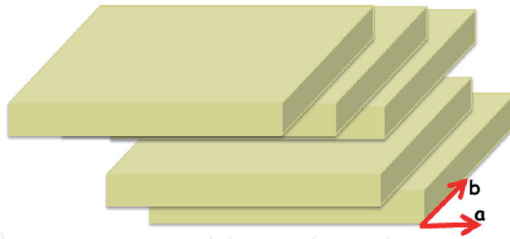
Figure 3. Disordered layers in the vermiculite structure.
