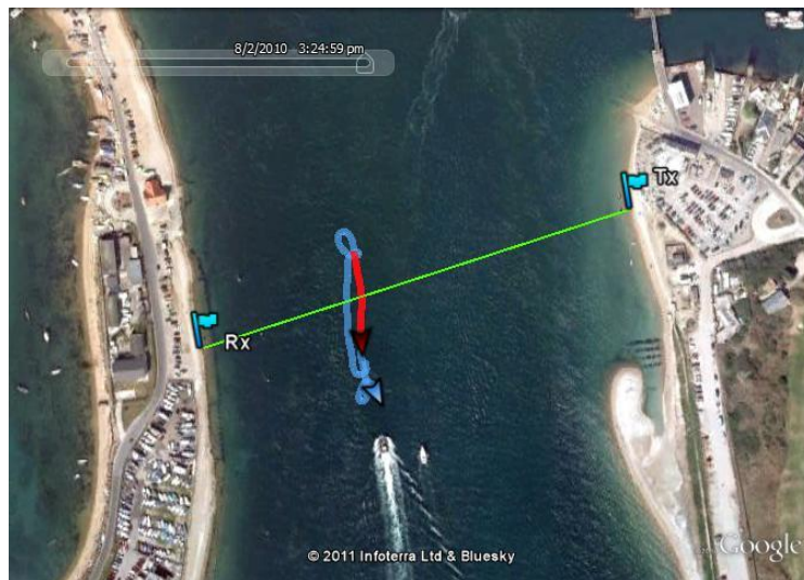
Figure 5.2.1 GPS track data for target trajectory. Blue shows full track and red indicates section used for analysis
