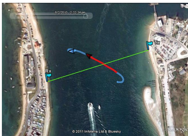
Figure 3.4.1 GPS track of the target crossing the FSR baseline forming a 52 degree crossing angle
