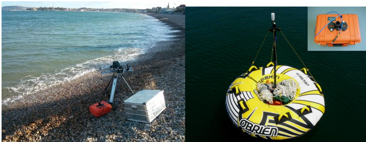
Figure 3.1.3 7.5 GHz transmitter placed on the shore using directional antennas mounted on a tripod (left) and 7.5 GHz transmitter mounted on a 60 inch Ringo (right)
