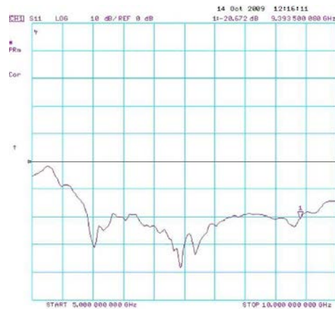
Figure A15 Measured S11 of the final horn (No2) antenna
