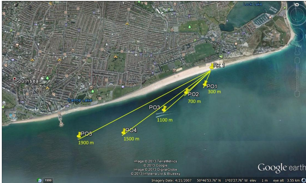
Figure 3.3.10 Location of the trial and the positions of the Tx and Rx
