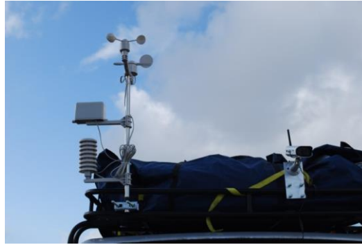
Figure 3.4.2 Weather station mounted on 3m poll
