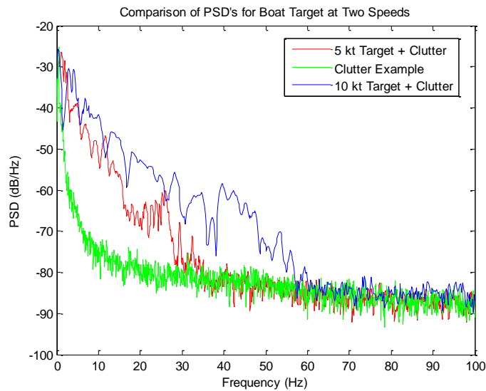
Figure 5.3.5 PSD comparison for boat target moving at speeds of 5kt and 10kt
