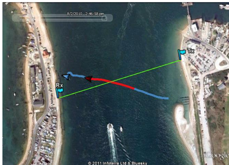
Figure 5.2.7 GPS track data for target trajectory. Blue shows full track and red indicates section used for analysis
