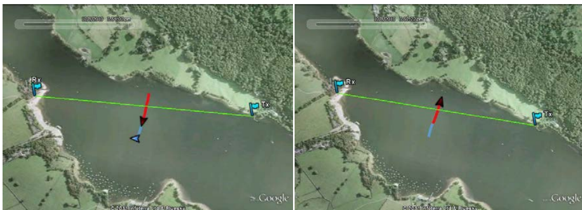
Figure 5.6.12 GPS track data for target trajectory's, left is for target signature in Figure 5.57 right 5.58. Blue shows full track and red indicates section used for analysis
