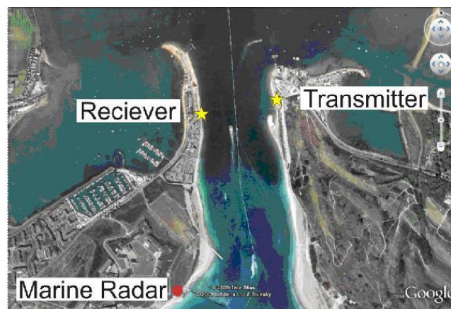
Figure 4.3.6 Topology of the sea trial test site
