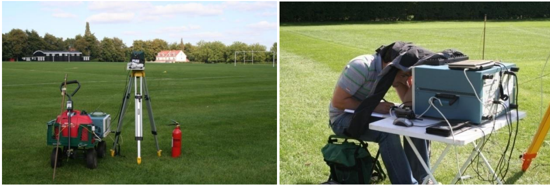
Figure 3.2.4 Sports field power budget measurements: a) AWG, generator and transmitter. b) receiver, scope, Doppler receiver & generator
