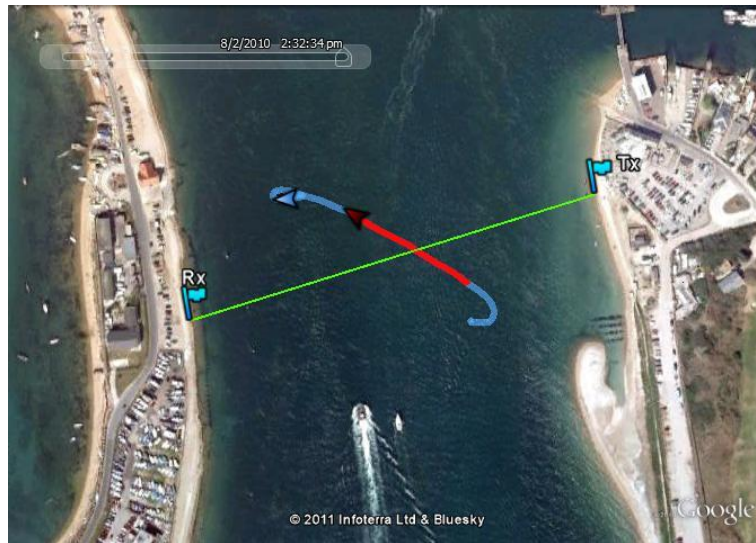
Figure 5.2.4 GPS track data for target trajectory. Blue shows full track and red indicates section used for analysis
