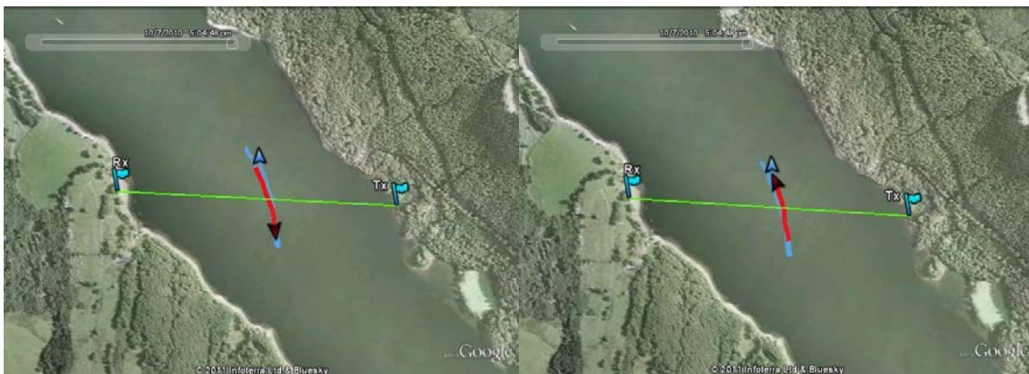
Figure 5.6.8 GPS track data for target trajectory's, left is for first target signature right for second. Blue shows full track and red indicates section used for analysis
