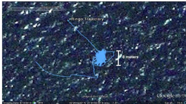
Figure 3.1.4: Six hour GPS track of the anchored Ringo tube in open sea
