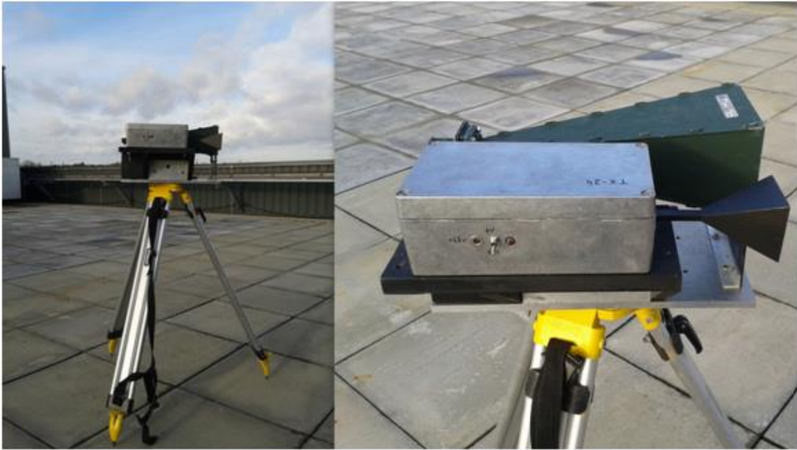
Figure 3.1.6 24 GHz FSR transmitter mounted next to the 7.5 GHz Tx
