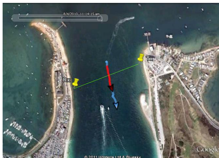
Figure 5.3.4 Map showing the measured target trajectory for the signature in Figure 5.3.3
