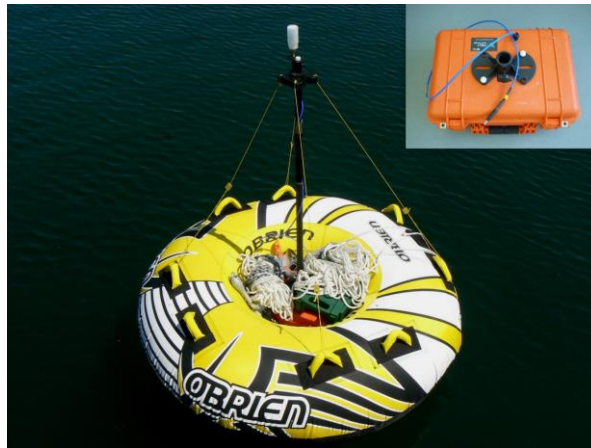
Figure A24 7.5 GHz transmitter mounted on a 60 inch Ringo. Attached are 2 anchors with 40m. of rope on each
