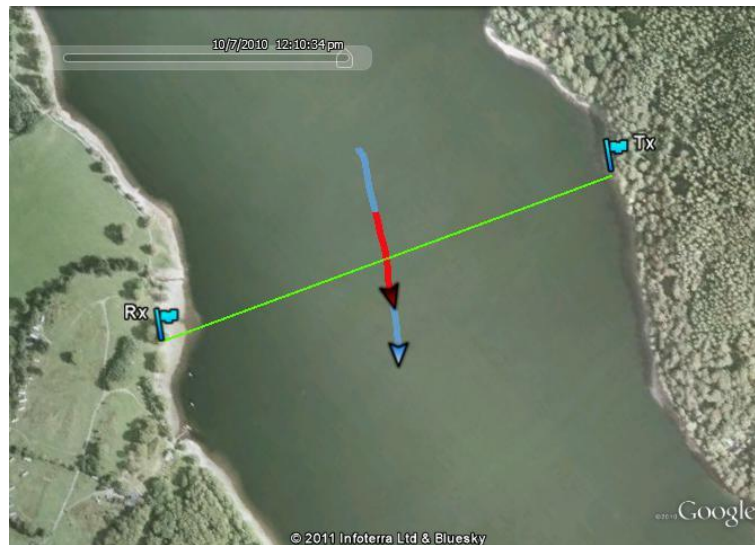
Figure 5.6.2 GPS track data for target trajectory. Blue shows full track and red indicates section used for analysis
