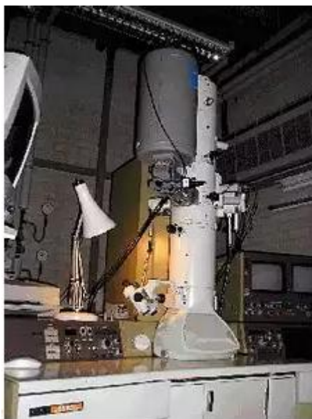
Figure 2.5 Jeol 1200EX TEM used in this project (courtesy of Centre of Electron Microscopy, University of Birmingham)
