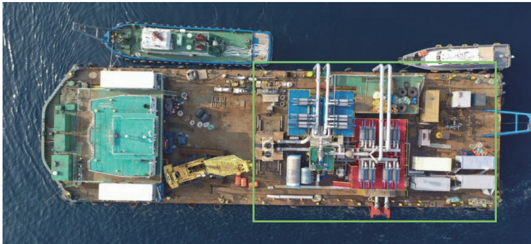
Figure 20. K-OTEC1000 plant onboard a barge ship in the eastern seas, near Busan, South Korea. The full extent of the OTEC plant is shown within the box in the figure. The plant was successfully tested in September, 2019, and it will be transported to South Tarawa in 2020 (Photograph: Kim).
