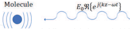
Figure 2. The mechanical response of the material to incoming monochromatic EM radiation. The vibrational response of the molecule is a function of its properties. This same principle is also related to the color of the flame that a molecule produces [1].
