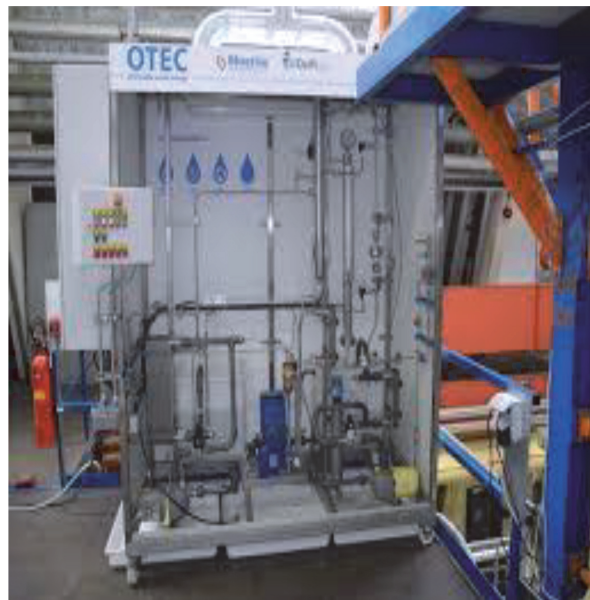
Figure 1. Experimental equipment of OTEC using the Kalina cycle (Bluerise).
