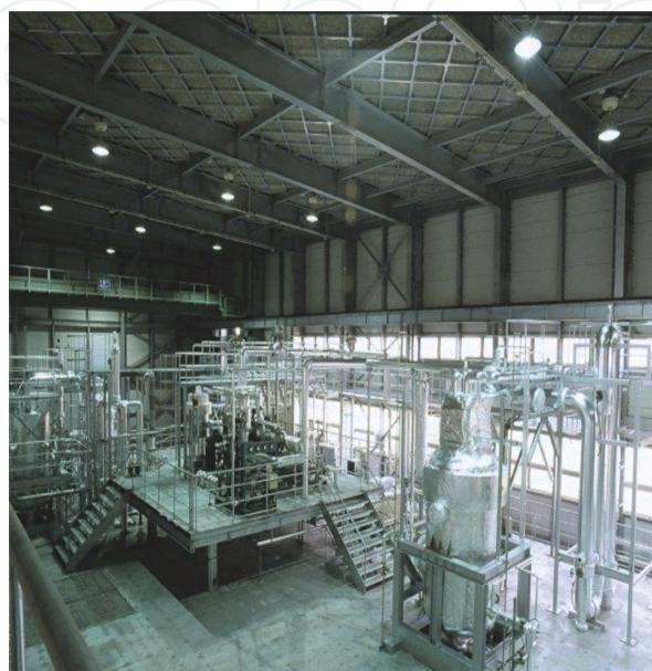
Figure 2. 4.5-kW experimental equipment of OTEC using the Uehara cycle (Saga Univ).
