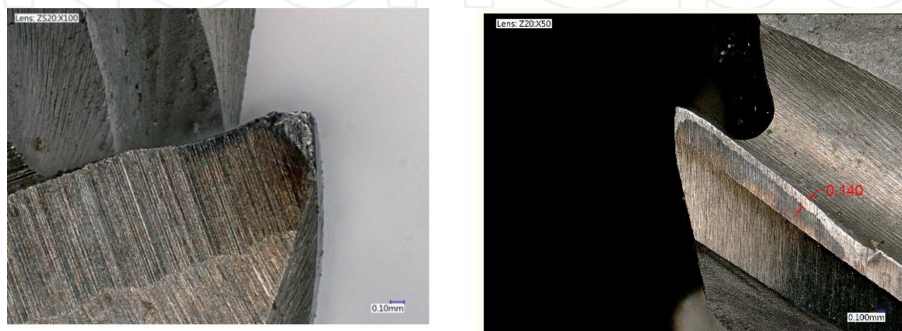
Figure 9. Notch wear and flank wear ( V_c = 30 m/min, soybean-based nanofluid) at 85 min [16].
