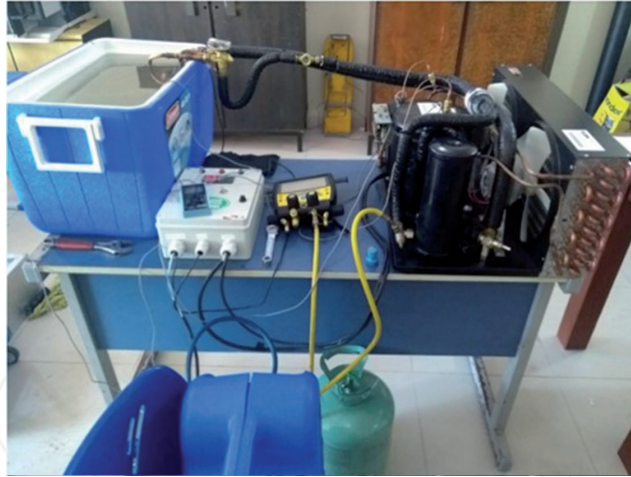
Figure 1. Bench tests with chiller mounted by ClimaTConT.
