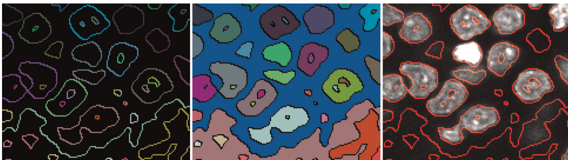
Figure 4. Connected components of the Laplacian operator's zero space. The boundary (left) is overlaid on the cell nuclei image (right). The connected components (center) are calculated from Laplacian of Gaussian, s = 12 .
