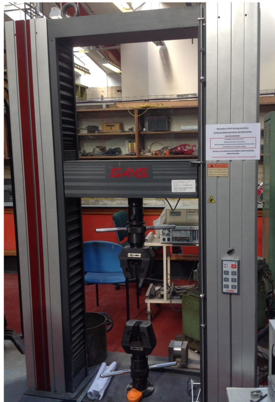
Figure A-1-1: Test device (SANS 20t test machine)
