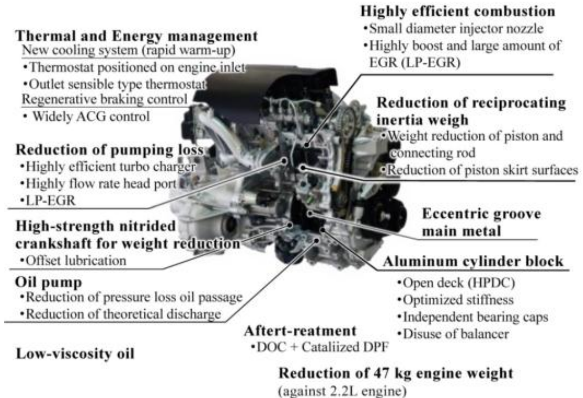
Figure 1-2 Key Technologies for Downsizing a Diesel Engine (Nishio et al. 2013)
