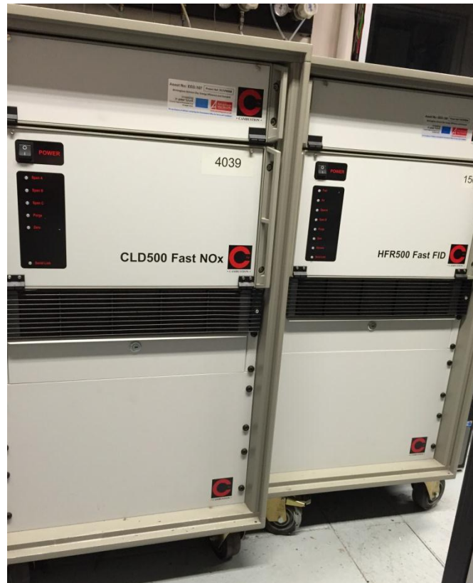
Figure 3-12 Cambustion CLD500 Fast NOx and HFR500 Fast FID Analyser
