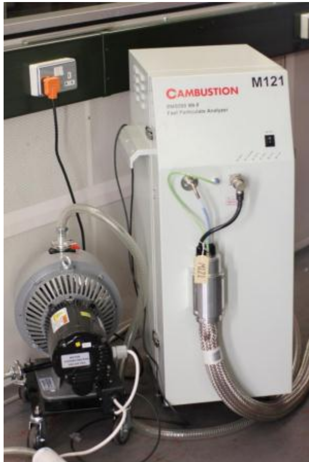
Figure 3-16 DMS500 Fast Particulate Spectrometer
