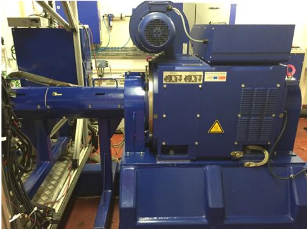
Figure 3-4 Transient Dynamometer in the Test Cell
