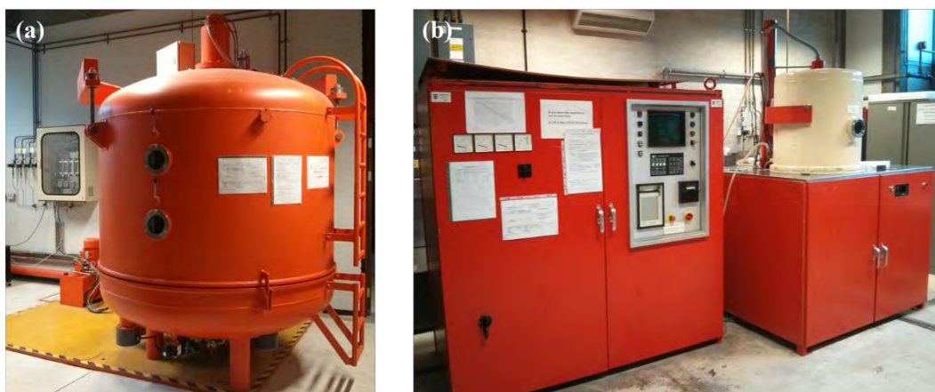
Figure 3.2.1 Plasma furnaces (a) AS Plasma Metal 75 kVA + 15 kVA industrial scale unit (b) DC Klöckner Ionon 60 kVA
