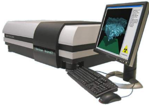
Figure 1.6: SkyScan 1172 micro-CT scanner (Bruker micro-CT). This particular instrument is commonly used in the biomedical sciences to image small tissue samples (e.g. teeth, bone). Software is supplied with the instrument for image acquisition, post-processing, reconstruction and visualisation. (Photograph reproduced from www.microphotics.com )
