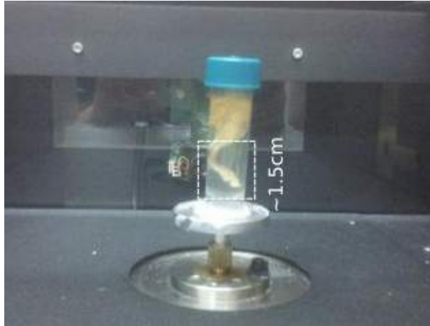
Figure 3.1: A hind paw sample, mounted in the micro-CT scanner. The dashed white box denotes the approximate field of view of the instrument.
