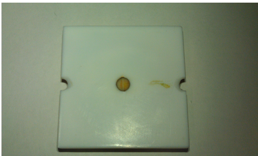
Figure 3.30: Discolouring of cement after prolonged contact with copper
