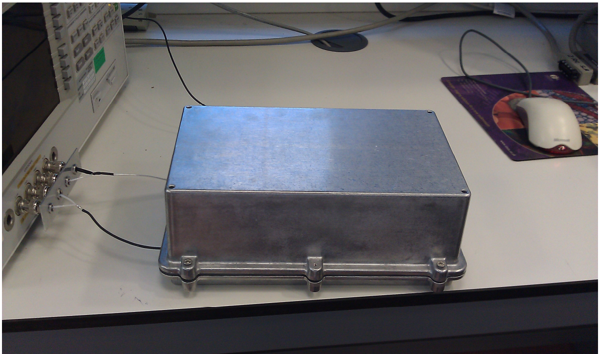
Figure 2.15: Co-planar assembly encased in grounded box to reduce interference from 50Hz frequency of mains power.
